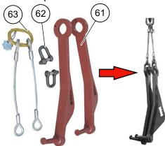
5. Lift the jaw into the vertical position and do a check of the lifting equipment. Do a visual inspection of the jaw lifting tool to make sure that it is secure on the jaw.
