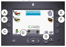
Pushing the crusher operation button on the main menu display screen will show the crushing mode display screen.
