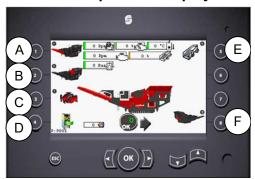
Pushing manual operation on the mode display screen will show the manual operation screen.
