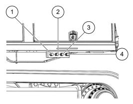
Look along the side of the machine for the fluid drain valves.
