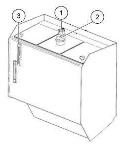
1. Use an applicable cleaning cloth to clean around the diesel fuel tank vent (1).
