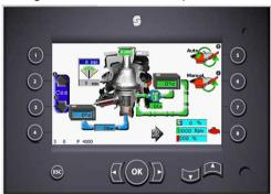
3. Push the [right arrow] button to go to the cone crusher level control screen
