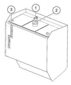
1. Look at the tank gauge (3) to do a check of the diesel level in the tank.
