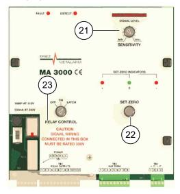
8. Adjust the sensitivity dial (21) to the minimum setting that will detect the test piece.
