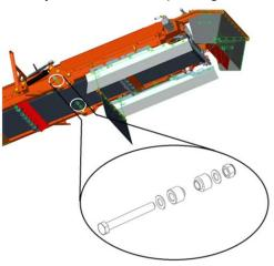
The stopper must be installed to prevent the conveyor head from impacting and damaging the attached MHS. The stopper is not required on short length main conveyors or on long length main conveyors which are not MHS ready.
