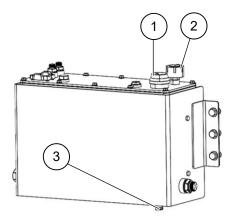
1. Look at the tank gauge to check the clutch oil level in the tank.
