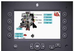
6. Push button [right arrow] 3 times to go to crusher calibration screen
