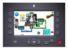
Adjust the closed size setting (CSS) setting by lifting or lowering the mantle.
