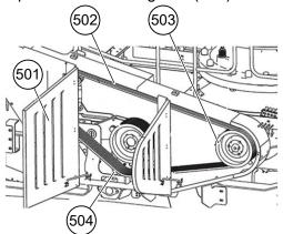
3. Loosen the locking nuts (505) on the tension adjuster (504).
