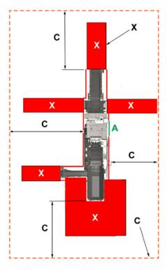
Put barriers 20m (65ft) from the machine to prevent access by personnel that do not operate the machine. There is a risk of mechanical hazards, material that can fall and ejected material.
