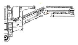
When the stopper is not installed, the conveyor will lower fully. Be aware that when the hydraulic system is deactivated, the conveyor head may drop until it touches the ground:
