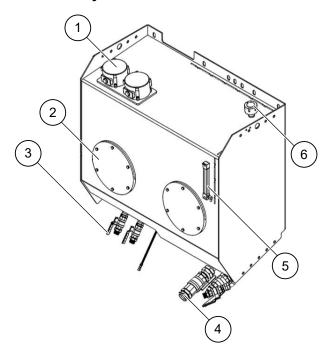
1. Look at the tank gauge (5) to do a check of the hydraulic oil level in the tank.
