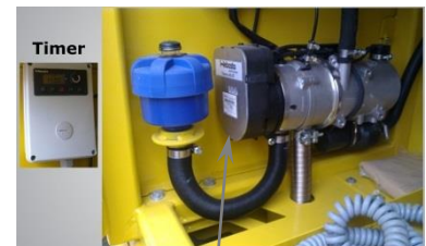
HEATING SYSTEM FOR ENGINE
